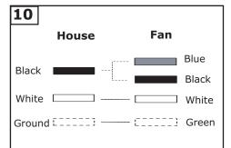
Connect black and blue wire from fan to Black or (Hot) wire from house. Connect White wire from Fan to White (Neutral) wire from house. Connect Ground leads from mounting bracket and downrod to Ground lead from house. Refer to Safety Tips section of manual.
